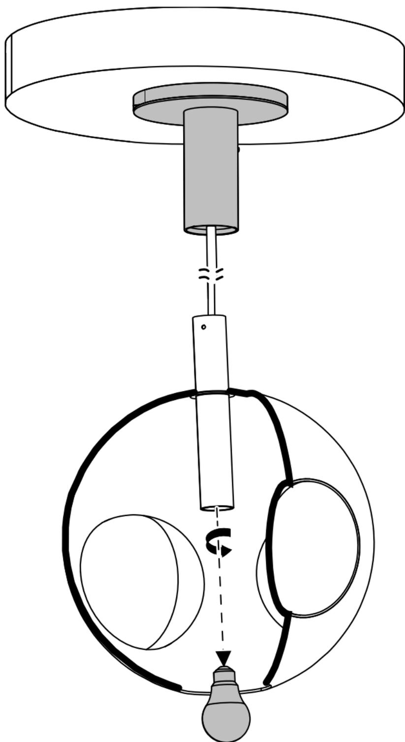
Carry out this step in reverse to fit the new bulb.
