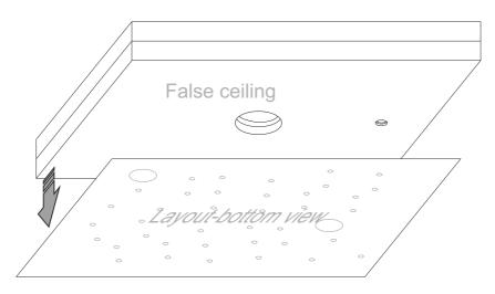
Step 4f/ Screw the screw anchors into all prepared holes.
