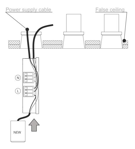
Step 9e/ Put the light source back in the ceiling.
