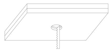
Step 4d/ Cut out the holes for the screw anchors. The number of holes varies from product to product. Follow the layout.
