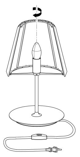
Screw the bulb in the socket clockwise. Use E14 bulb with the following specifications: max. 40W, 230V. The manufacturer shall not be held responsible for improper function when other light source is used.
