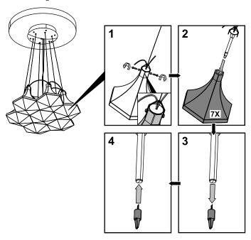
Carry out this step in reverse to fit the new bulb.
