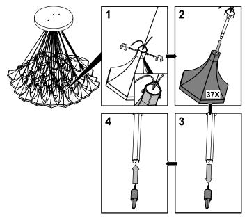
Carry out this step in reverse to fit the new bulb.
