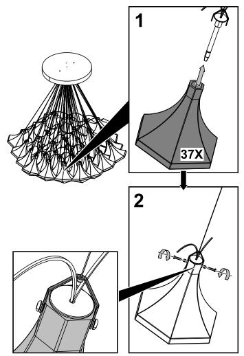
If you cannot align the glass components (detail B) in order to achieve desired shape (detail A), exchange some of glass components (detail A). The glass components are made from hand-blown glass, it contains small imperfections.
