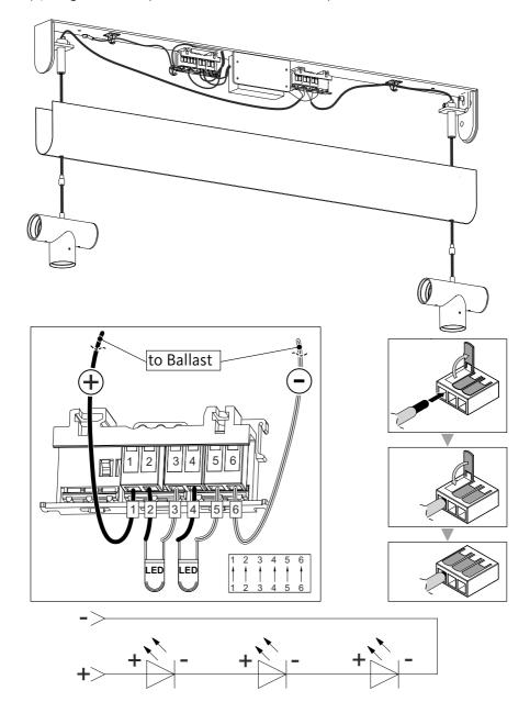
Step 9c/ Light source output - all constant current LED chips are serial connected
