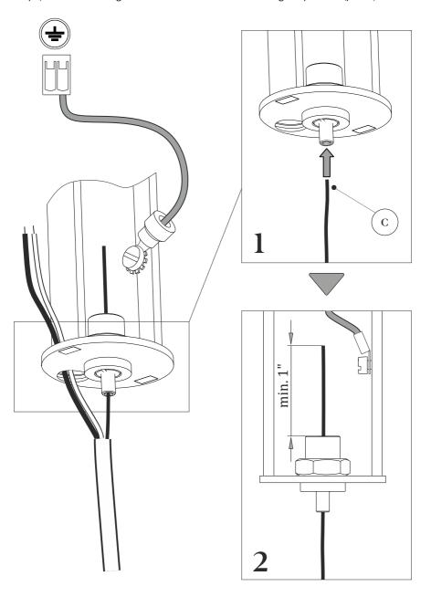
Step 4b/ Detail B for connection of mains input and light source output.
