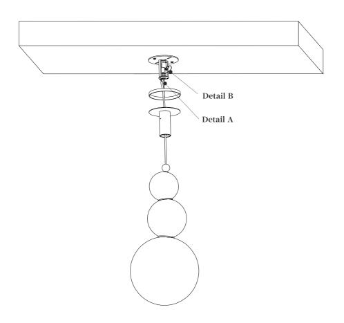
Step 4a/ Detail A for Light source cable - Wire cable securing the pendant (pos. C)
