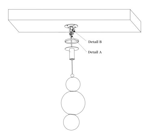
Step 4a/ Detail A for Light source cable - Wire cable securing the pendant (pos. C)
