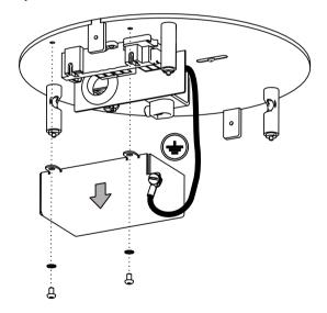
Step 4c/ Place the assembly with light source into the glass.
