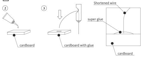
Excess glue must be wiped off immediately to allow further manipulation of the wire in the Reutlinger.
