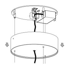
For easier installation use the included installation hooks (pos. A). Take care not to break the ground cable (pos. B).
