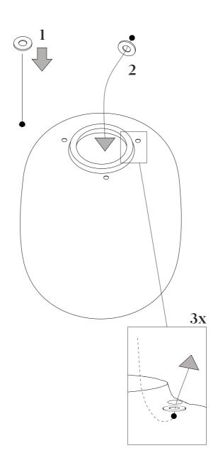
Step 3b/ For easier installation use the included installation hooks (pos. A). Take care not to break the ground cable (pos. B).
