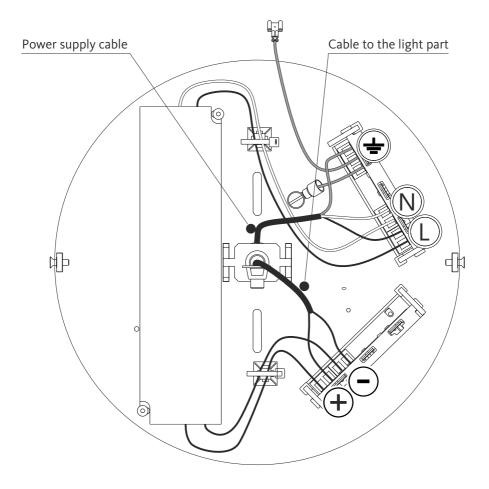
Step 7c.2/ Wiring for DALI dimming
