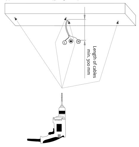
Step 5d/ Cut out the holes for canopy and glass component.
