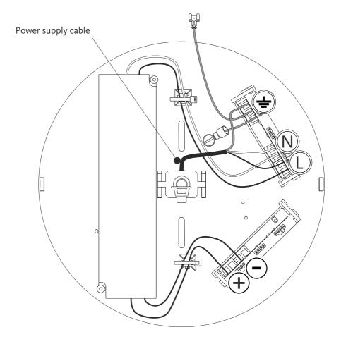
Step 7a.2/ Wiring for DALI dimming
