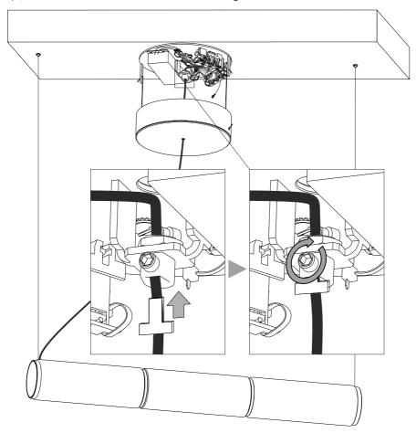
Step 7e/ Secure with a screw. Be careful not to damage the cable.
