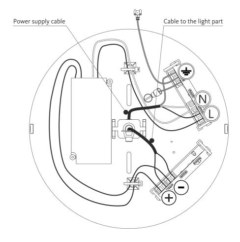
Step 7e/ Secure with a screw. Be careful not to damage the cable.
