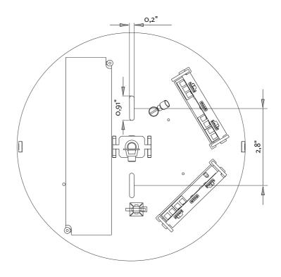
First prepare a 4" J-Box with 50 lb capacity and PE cable, then you can proceed with the installation.
